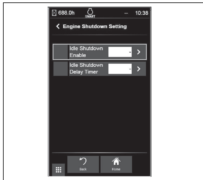
Figure 6-111: Engine Shutdown Screen
