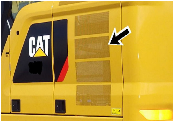
Figure 7-83: Radiator Compartment Door
