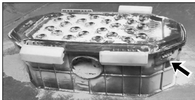
Figure 10-106: Pre-cleaner Locking Tabs
