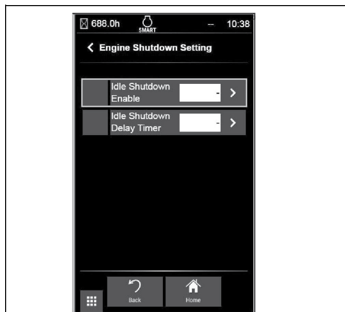
Figure 6-111: Engine Shutdown Screen
