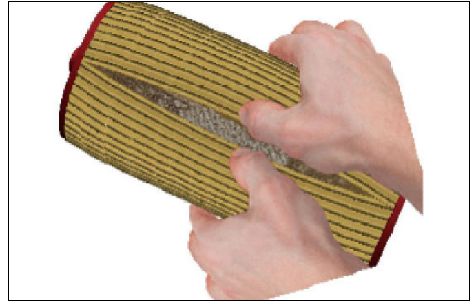
Figure 10-156: Hydraulic Oil Filter Inspection
