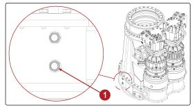
If the oil level is low, add oil. See Section: "Adding the Rotary Casing Oil " (page 513) for more information.
