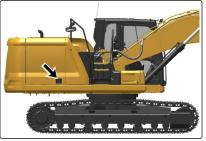
4. If the hydraulic oil temperature is between 31°-49° C (87° to 121° F), maintain the oil level in the lower half of the operational range. If the hydraulic oil temperature is between 50°-80° C (122° to 187° F), maintain the oil level within the upper half of the operational range. For temperatures from 10° to 30° C (50° to 86° F) maintain the oil level slightly above the lower limit.
