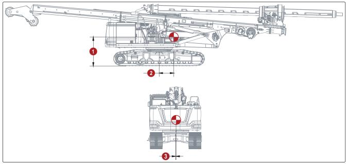
0000483 Center of Gravity-Transportation-Standard Mast
