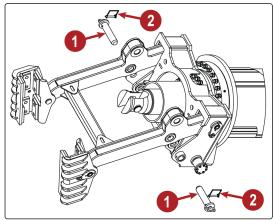
12. Using a rubber mallet, strike the two lock pins on the A-frame to remove them from the A-frame assembly.
