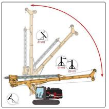
9. Make sure the A-frame (8) is below the detent (9) on the mast. Lower the rotary (10) as required.
