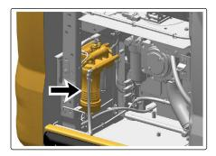
2. Turn drain valve (4) counterclockwise to open. The drain valve is on the bottom of the water separator. Refer to *Containing Fluid Spillage\** (page 84) for more information.
