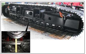
4. Add grease through injection valve (1) to reduce the clearance between the track roller and track link. Loosen injection valve (1) to increase the clearance between the track roller and track link.
