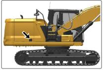
2. Open drain valve (1) on the bottom of the fuel/water separator element. Drain the water into a suitable container.
