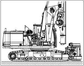
3. Remove the mast lock assemblies from both sides of the foot mast.
