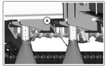
3. Find the center track roller. Measure the clearance between the top of the track chain link and the bottom surface of the track roller where the link rides. Refer to *Specifications (page 494)* for the correct dimension for your undercarriage model.
