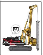
9. Raise the kelly bar to the top of the mast so it clears the top of the rotary.
