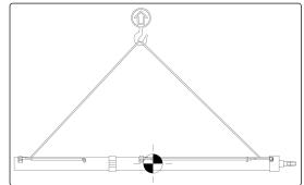
9. Hook the long mast assembly (head mast, upper mast, and mast extension) with an appropriate lifting device. Beware of the center of gravity.
