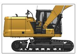
2. Remove drain hose (3) from the holder (1) on the upper frame. Face the end of the hose toward the container. Refer to *Containing Fluid Spillage\* (page 84)* for more information.
