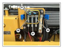
Spare (51) – The fuse module includes spare fuses which can be used if one of the installed fuses opens. One spare fuse is provided for each fuse in use.
