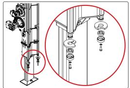
c. Remove the lock bolt and crowd cylinder rod pin to disconnect the crowd cylinder from the rotary. If necessary, slightly move the crowd cylinder to facilitate the removal of the pin.
