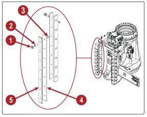
0000361 Rotary Head-Sled Wear Pad Removal-Installation Procedure
