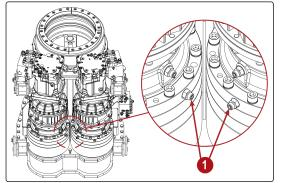
7. If the oil level is low, add oil. See Section: "Adding the Rotary Reducer Oil " (page 510) for more information.
