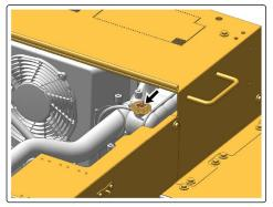
5. You may need to drain some coolant from the radiator so that a coolant extender can be added to the cooling system.
