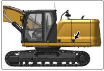
Open the drain valve and allow the coolant to drain into a suitable container. The drain valve is on the bottom 6. of the radiator. Properly dispose of used coolant.
