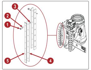
0000361 Rotary Head-Sled Wear Pad Removal-Installation Procedure
