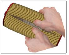
g06224663 Hydraulic System-Oil Filter Inspection
