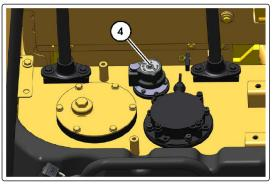
7. Release the pressure that may be present in the return hydraulic circuit with the following procedure. Refer to Illustration for filler cap positions.
