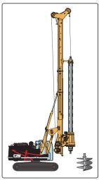
2. Move the drilling rig to align the kelly bar with the work tool.
