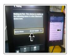
Note: The device name on your phone should be "##CAT RADIO", with the number being from "00" to "99".
