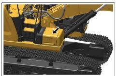
2. Ensure that the area around the DEF filter is clean and free from dirt. For clarity, the DEF assembly has been removed from the compartment.
