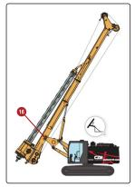
20. Tilt the mast backward. While lowering, make sure it is aligned with the chassis by operating both mast-tilting levers at the same time. Use an individual mast tilt lever to adjust the alignment as needed.
