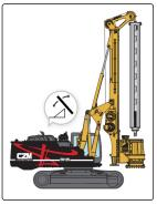
11. Attach a guide rope to the kelly bar and have an assistant guide the kelly bar into the rotary.
