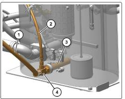
g06220559 Hydraulic System-Drain Filter
