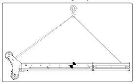
14. Install the long mast assembly on the main mast.
