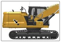
2. Open the drain valve by turning the valve counterclockwise. Allow the water and the sediment to drain into a suitable container.
