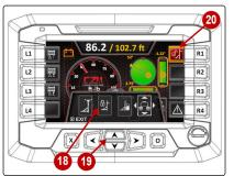
19. Use the down arrow button (19) or touch near the down arrow (21) on the display to unlock the detent arm. When unlocked, the R1 unlock icon (20) will illuminate.
