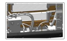
Obtain the sample of the coolant as close as possible to the recommended sampling interval. To receive the full effect of  $S \cdot O \cdot S$  analysis, a consistent trend of data must be established.
