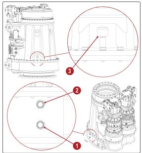
0000285 Rotary Head-Casing Adding Oil Procedure
