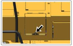
16. Remove oil filler cap (2). Fill the crankcase with new oil. See Section: "Fluids and Lubricants" (page 398). Clean the oil filler plug and install the oil filler plug.
