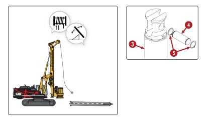
10. Return the mast to the vertical position and wind up the wire rope to a safe height.
