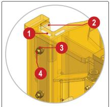
0000204 Rotary Head-Sled Wear Pad Adjustment Procedure
