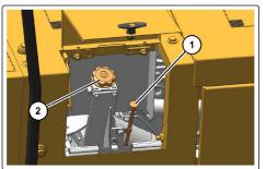
3. Remove the dipstick and check the dipstick. The oil level should be between the "L" mark and the "H" mark.
