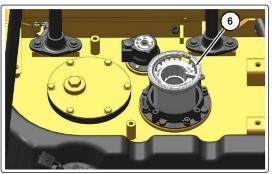
8. Place cover assembly (5) into position in the tank. Install bolts (4) and tighten to  $30 \pm 7$  N·m (22  $\pm 5$  lb-ft). Install the harness connector on the filter bypass switch.
