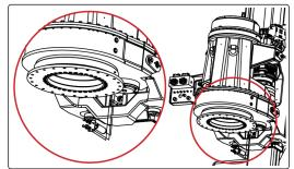
d. Use the forklift to lower the rotary until the mast is above the rotary.
