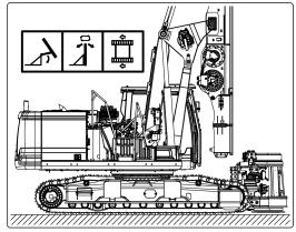
5. Align the crowd cylinder rod end with the rotary head. Install the rod pin and fasten the lock bolt to secure the crowd cylinder to the rotary sled. If necessary, slightly move the crowd cylinder to facilitate the installation of the pin.
