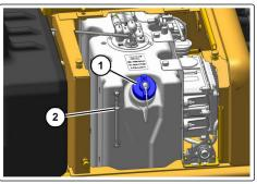
2. Remove the blue DEF tank filler cap (1).
