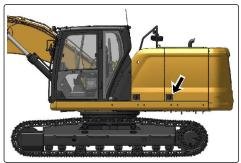
2. Inspect the condenser for debris. Clean the condenser, if necessary.
