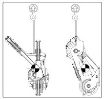
8. Remove the connection bolts between the mast head and the mast.
