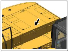
2. Remove the lid that holds the canister to the filter base assembly.
