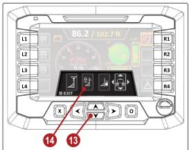
15. Use the down arrow button (13) or touch near the down arrow (15) on the display to place the A-frame detent arm in the unlocked position.
