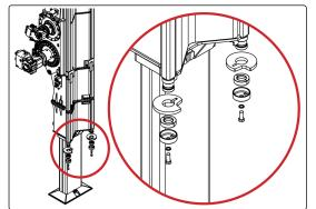
7. Connect the hydraulic lines to the rotary sled manifold. Use tags made during disassembly for identification of connections.
