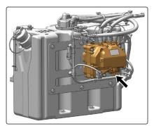
3. Unscrew the cap, and remove the expansion device (1) from DEF filter (2).
