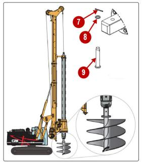
3. If the work tool is possibly unstable, add support to prevent tipping when the kelly bar is removed.
