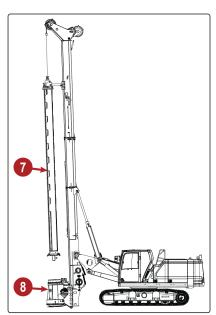
7. Lower the kelly bar using the main winch until the bottom of the kelly bar (12) rests on the ground. Tilt the mast forward as needed to keep the kelly bar from contacting the rotary head (13).
