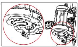
d. Slowly raise the mast and at the same time move the machine forward until the mast is above the rotary. Maintain the "auto-tilt" function activated throughout this step to ensure that the mast remains vertical.
