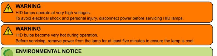
Although HID bulb materials may change over time, HID bulbs produced at the time of the printing of this manual contain mercury.
