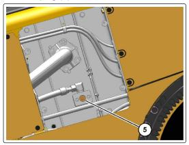
10. Inspect the O-ring. Replace the O-ring if wear or damage is evident.
