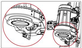
6. Install the mast lock assemblies on both sides of the foot mast.
