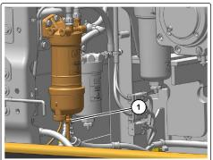
3. Close the drain valve when all the water has been drained.
