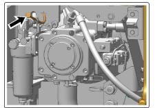
g06211545 Engine Oil Level-Ground Level Dipstick
