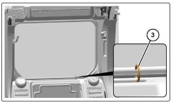
g06187008 Alternate Exit-Rear Window with Ring Seal
