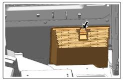
3. Slide the filter element upward.
