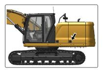
4. Check the coolant reservoir. Maintain the coolant level so that coolant is between the "ADD" and "FULL" lines. If more coolant is needed, see Section: "Adding the Cooling System Coolant Extender (ELC)\*" (page 427).
