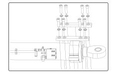
8. Use an appropriate lifting device to remove the crowd cylinder. Attach two lifting points to the ends of the components and beware of the center of gravity of the components.
