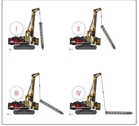
6. Turn off the bottom-hole system to allow the main winch cable to be unwound without any tension on the cable.
