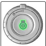
g06226444 MSS-Engine Start Switch MSS Disarmed or Uninstalled
