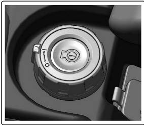
g06215426 MSS-Engine Start Switch with Integrated MSS Indicator
