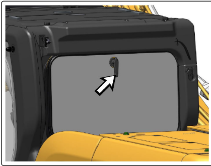
g06213471 Alternate Exit-Rear Window with Lever 2
