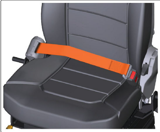
g06223894 Releasing The Seat Belt
