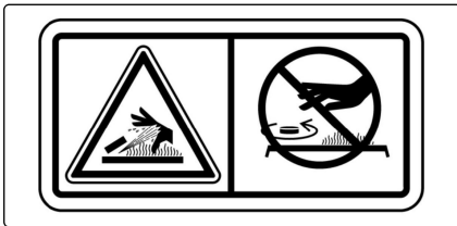
g01371640 Relieve Hydraulic Tank Pressure
