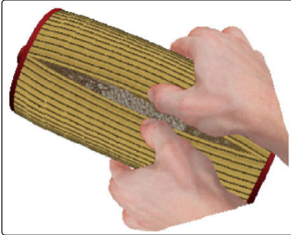
g06224663 Hydraulic System-Oil Filter Inspection
