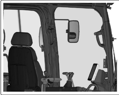
g06223277 Mirrors-Right Side View Mirror on the Cab
