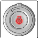
g06226442 MSS-Engine Start Switch MSS Armed
