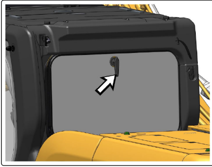
g06213471 Alternate Exit-Rear Window with Lever 2
