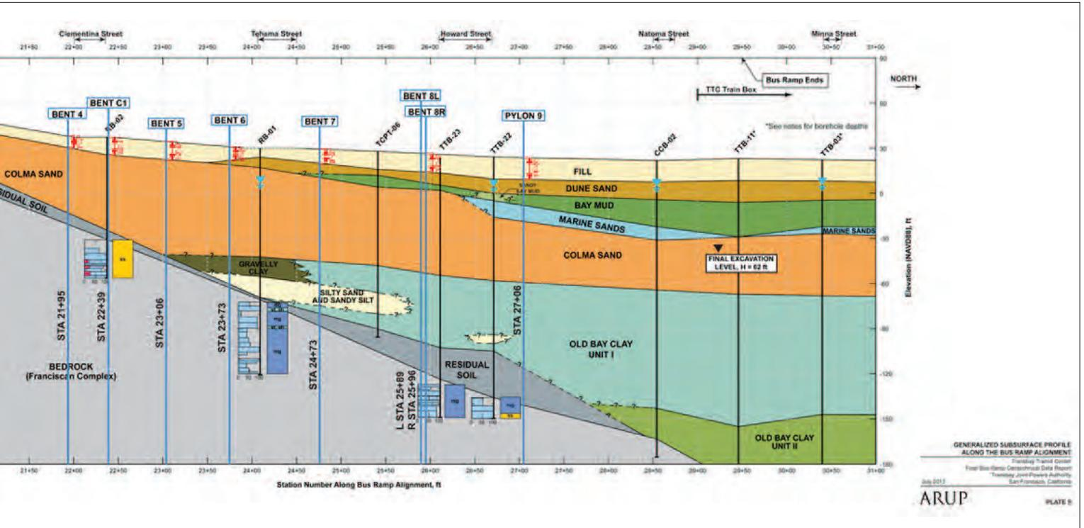
a sequence of sediments, including fill, dune sand over Bay Mud, which overlies marine sands and Colma Sand, followed by the Old Bay Clay, sometimes over residual soil over bedrock. The soil deposits at the southern end of the project consist of fill over bedrock to approximately Harrison Street. South of Harrison Street, the subsurface strata consist of fill, Colma Sand, and residual soil over bedrock.
