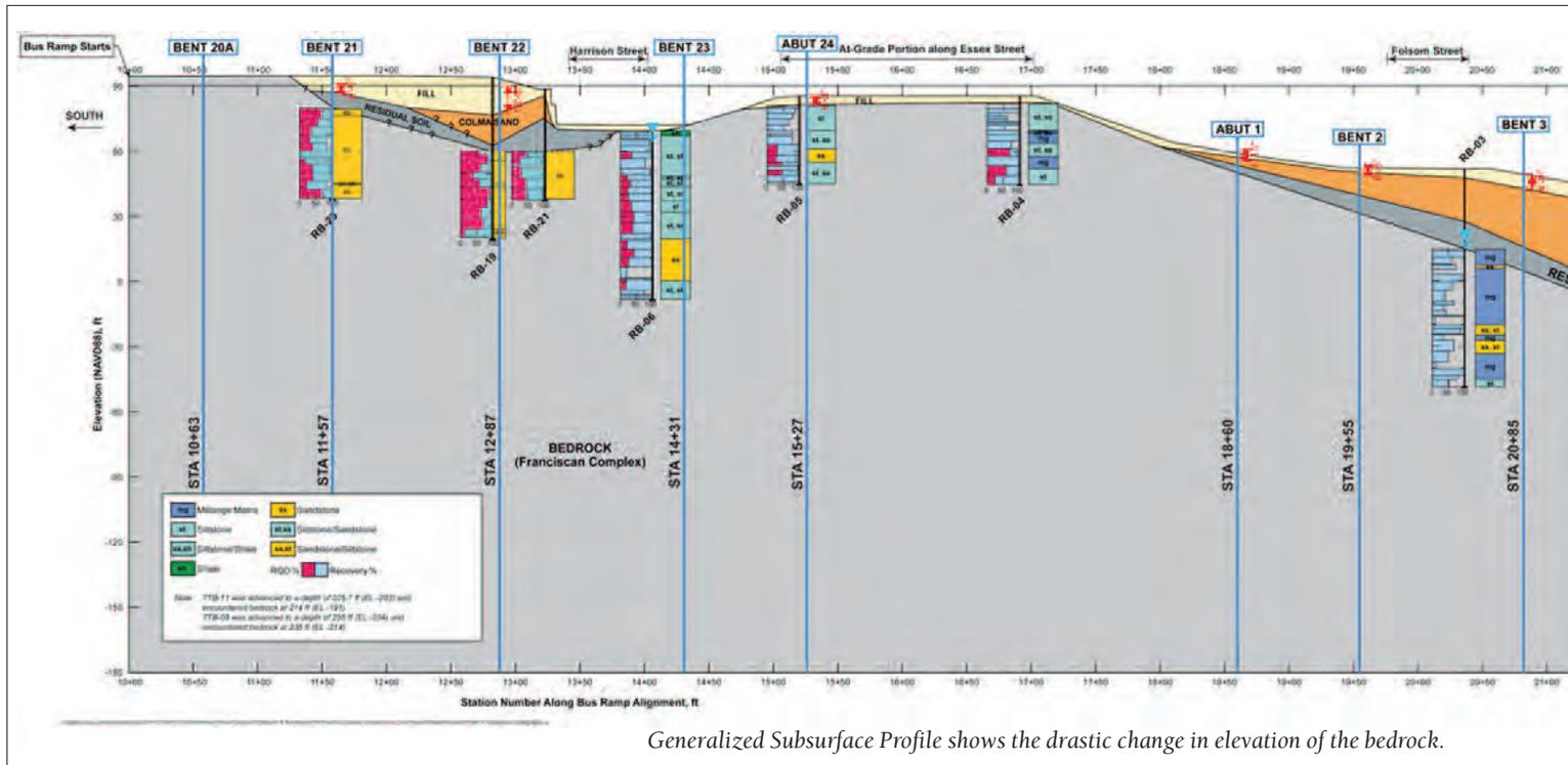
Generalized Subsurface Profile shows the drastic change in elevation of the bedrock.
