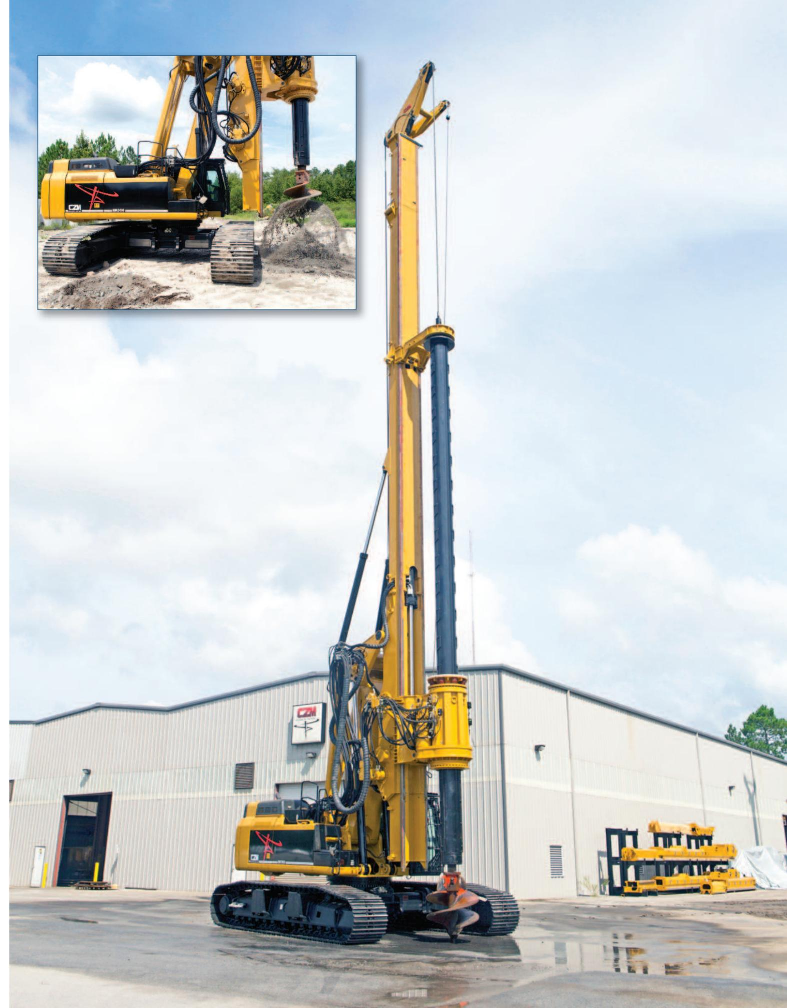
The EK300 is also the answer to numerous requests for a machine strong enough to build Secant Pile walls, installing European style casing deeper than 100 feet and with diameters of more than 4 feet. Its weight, torque and pulling force make the EK300 the ideal machine for this application. Its 21.3 feet of crowd/pull-up stroke allows the contractor to work with 20-foot casing sections, significantly increasing job productivity.
