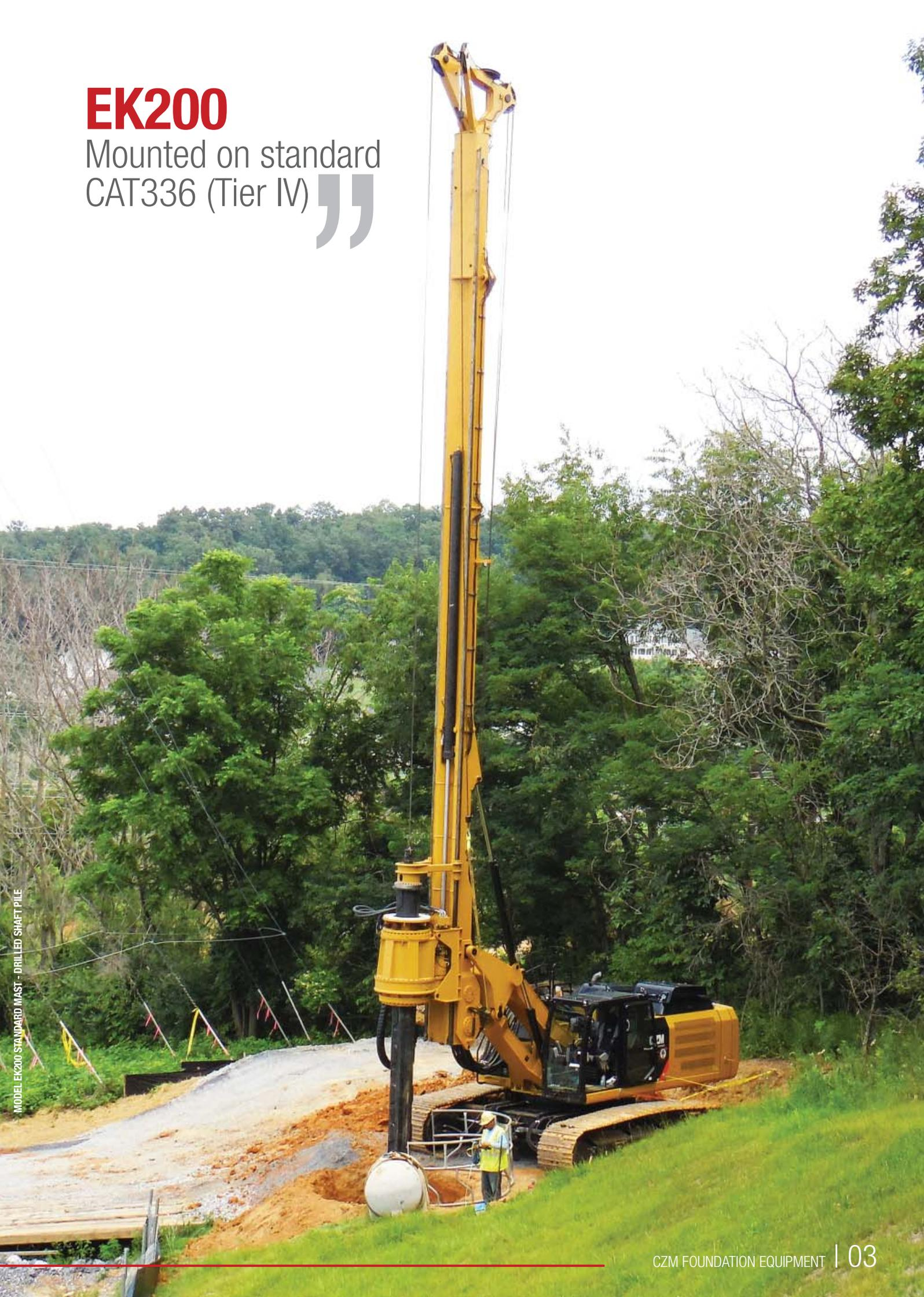
MODEL EK200 STANDARD MAST - DRILLED SHAFT PILE
