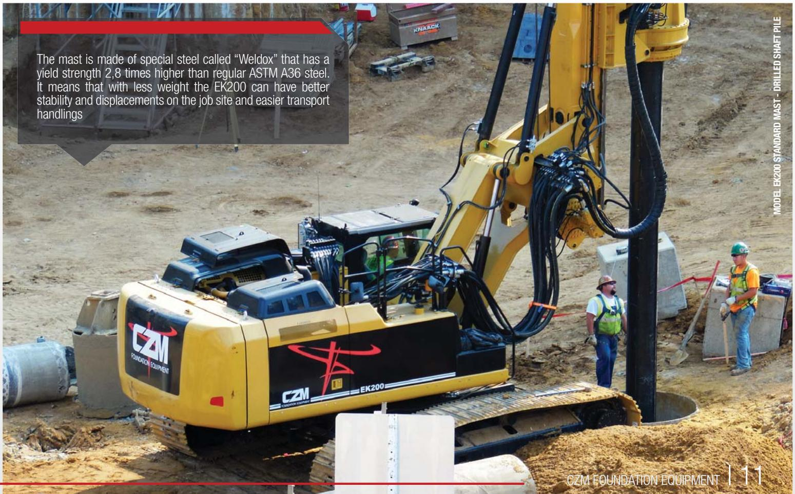
The mast is made of special steel called "Weldox" that has a yield strength 2,8 times higher than regular ASTM A36 steel. It means that with less weight the EK200 can have better stability and displacements on the job site and easier transport handlings
